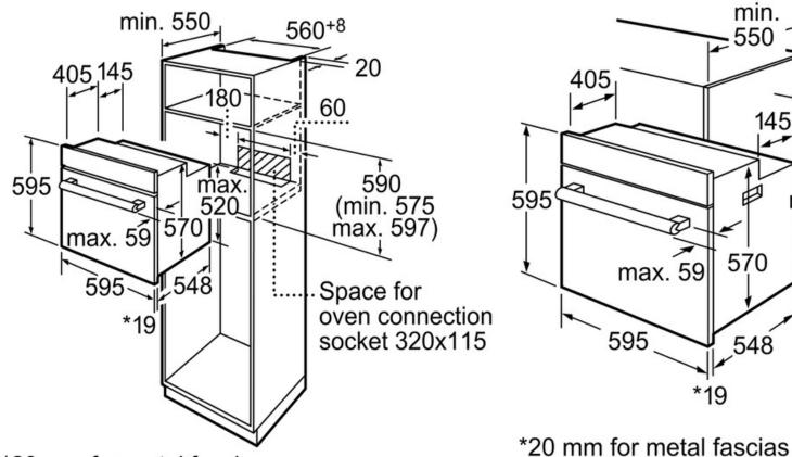
,□ max. 20 min. 560+8 550 405 180 -16<u>0</u> 595 600+4 570 max. 59 595 Space for oven 548 connection socket \*19 320x115
