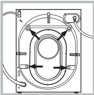
3. Remove the 4 protective screws and the rubber bush with the respective spacer, situated on the rear of the appliance (see also the installation leaflet). NB: The plastic spacers may fall down inside the machine once the bolt has been removed, and
