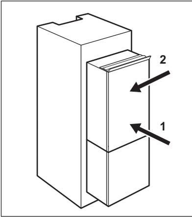
4. Push the appliance in the direction of the arrows (2) against the cupboard on the opposite side of the hinge.
