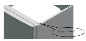
3. Remove middle hinge, screws, screw caps and plastic inserting nails. Install them on the other side. Take off the lower door and put it away.
