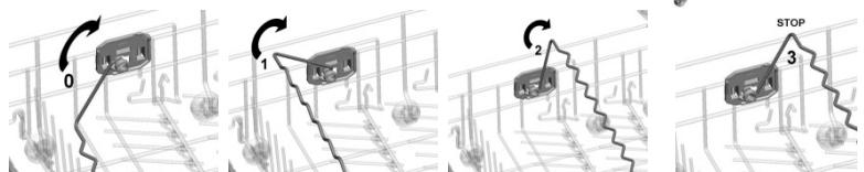
2-position fold-down supports (1-2). In position 1 (vertical) they can be used to take plates, while in position 2 (slanted) they provide support for long-stem glasses which will be held in place by the **glass holder**. Adjustment: raise point **P** as shown until the support turns into position 2.
