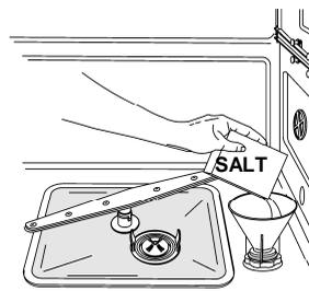
When using water of medium hardness, the regenerating salt container should be refilled after approximately **20 washing cycles**. The salt container can hold approximately **1.7 Kg** of salt in grains. The container is situated at the bottom of the dishwasher. After removing the lower basket, unscrew the salt container cap by turning it anticlockwise and pour in the salt using the funnel supplied with the dishwasher. Before replacing the cap, remove any salt residues from around the opening.
