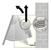
After installing the extractor hood, insert the activated carbon filter.
