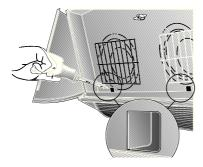
**5.** Insert activated carbon filter in the lower left corner of the housing. Shift it until both hooks slot into the holes and then secure in place with the wing nut.
