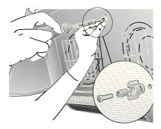
4. Using a screwdriver or similar, press the two lugs in the housing through to the back (only necessary upon initial fitting).
