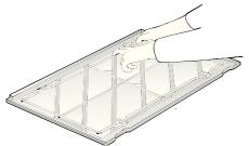
2. Position the filter screen against the housing and push upwards. Push in the lower edge over the lugs and lower the grid into place.
