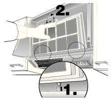
6. Position the filter screen against the housing and push upwards. Push in the lower edge over the brackets and lower the screen into place.
