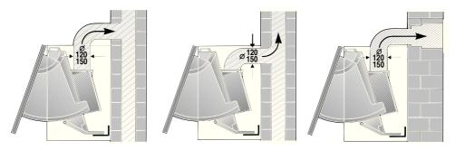
The exhaust air is discharged upwards through a ventilation shaft or directly through the outside wall into the open.
