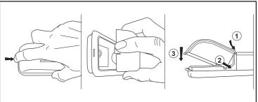
Unscrew the bulb to remove it from the socket. Replace the bulb with another having the same characteristics (LED S25-E14, max 1.4 W), screwing the new one into place.
