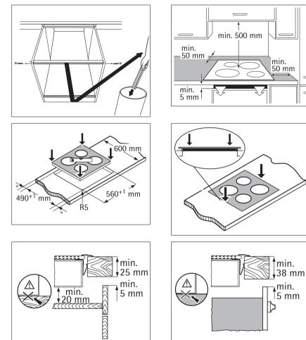
If you use a protection box (additional accessory), the front ventilation space of 5 mm and protective floor directly below the appliance are not necessary.
