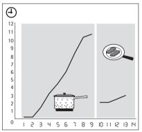
You can get a necessary heat setting in a shorter time if you activate the Automatic Heat Up function. This function sets the highest heat setting for some time (see the graphic), and then decreases to the necessary heat setting.
