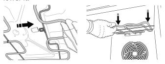
**2.** To return the heating element to its position, lift it up, pull it slightly towards you and make sure that the tab support is in its proper seating.
