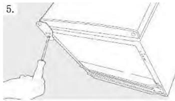
5. Slide the Appliance door back on to the top hinge making sure it's the right way up. Screw the bottom hinge into place on the new side.
