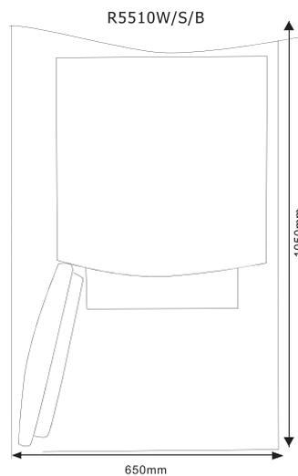
when the product is reversed you need to open the door to 650mm to enable you to open the Freezer Compartment Door.
