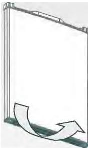
4. Unscrew the three screws on the down hinge and screw them on the opposite side.
