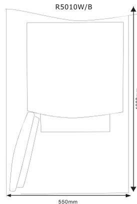
when the product is reversed you need to open the door to 550mm to enable you to open the Freezer Compartment Door.
