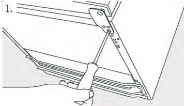
1. Undo the screws and remove the hinge bracket from the base. A spanner may be required to loosen the bolts first.
