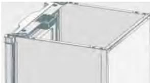
b: Move the shaft sheath and block piece to opposite side also
