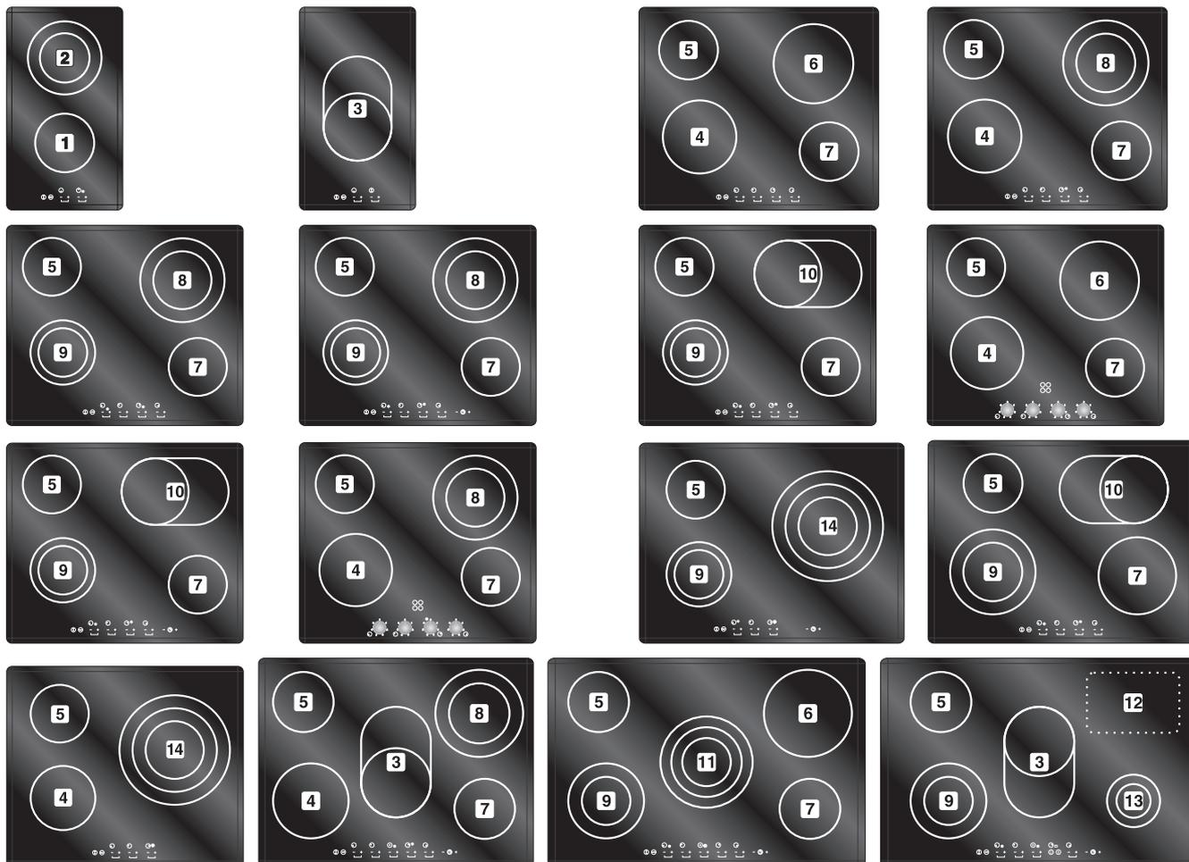
The appliance features 4/5 cooking zones of different diameter and power. Their position is clearly indicated by circles and the heat given off is defined by the markings on the glass surface. The 5 cooking zones are of the HIGH-LIGHT type and come on after a few seconds of being activated. Heating intensity can be adjusted by means of the knobs located on the front panel from a minimum setting of 1 to a maximum setting of 6/9 (Depending on models).
