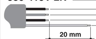
**For operation on 220-240 V 3~:** use an - H05V2V2-F type four-core cable (4 x 2,5 mm<sup>2</sup>).
