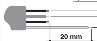
**For operation on 220-240 V~:** use an - H05V2V2-F type three-core cable. (3 x 4 mm<sup>2</sup> : hob with 5 cooking zones)
