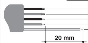
**For operation on 380-415 V 2N~:** use an - H05V2V2-F type four-core cable (4 x 2,5 mm<sup>2</sup>).
