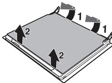
3. Some models have an intermediate glass pane. Remove the intermediate glass pane by lifting it upwards.
