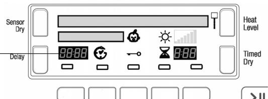
The display counts down the minutes of the delay period after the Start/Pause button is pressed.
