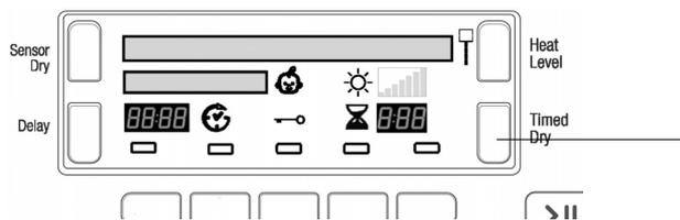
After selecting a programme that has a Timed Dry option, press the Timed Dry button and the display will increment the selected time, each time you press and release the button (see *Start and Programmes*).
