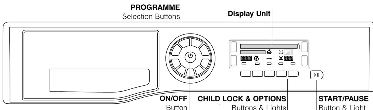
The **ON/OFF** button
