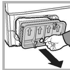
Release the three catches by turning 90° counter-clockwise then pull on the grip and remove from the dryer.
