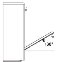
Grasp the door on both sides with both hands, lift it forming an angle of around 30° and remove it.
