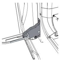
Open the door completely. Insert a pin into the hole in the hinge. Repeat for both hinges.
