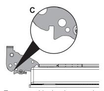
To reassemble the door, put the hinges in the relevant slots in the oven, making sure that grooved sections C are resting completely at the base of the slots. Lower the door and once it is in place remove the pins from the holes in the hinges.
