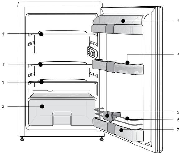
7. To tilt a shelf place the back of the shelf one level below the front of the shelf. To remove a tilted shelf, first release the back off the grooves and then pull it.
