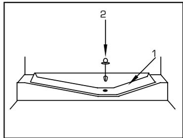
check to ensure that no food particles have blocked the drain tube. The drain tube can be cleared by pushing the special plastic plunger provided down the drain tube.
