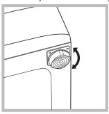
1. Install the washer-dryer on a flat sturdy floor, without resting it up against walls, cabinets or anything else.
