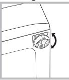
Your machine may make a considerable amount of noise if the two front feet have not been adjusted correctly. 1. Install the washing machine on a flat sturdy floor, without resting it up against walls, cabinets or anything else. 2. If the floor is not perfectly level, compensate for any unevenness by tightening or loosening the adjustable front feet (*see figure*); the angle of inclination, measured according to the worktop, must not exceed 2°.
