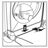
2. make sure the water level inside the machine is lower than the door opening; if it is not, remove excess water using the drain hose, collecting it in a bucket as indicated in the figure. 3. remove the cover panel on the lower front part of the washer-dryer (see figure).
